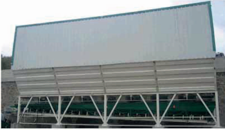
1-2- Aggregate Bunker, Weigh Conveyor and Plate
